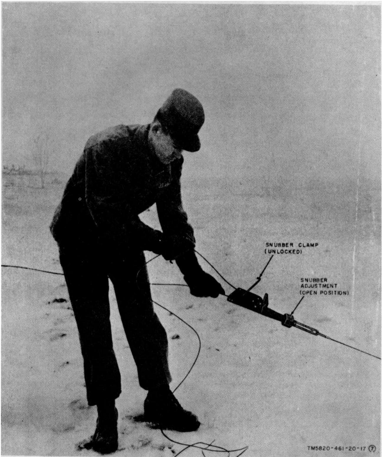
Figure 2-17(7). Erection of launcher (part 7 of 9).
